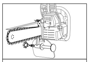
STEP 4 Insert axle into the mounting bracket as shown and firmly tighten knob
