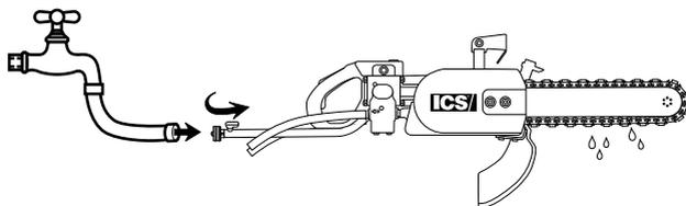
Attach to water supply capable of delivering 1.5 bar (20 psi) pressure to the power cutter at a minimum flow rate of 4 lpm (1 gpm). The single most important factor an operator can control to increase chain life is to use adequate water pressure.
