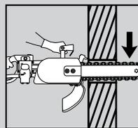
3. Insert WallWalker® rotate rear handle up, to rotate the nose down
