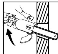
4. Rotate rear handle down, to rotate the nose up.
